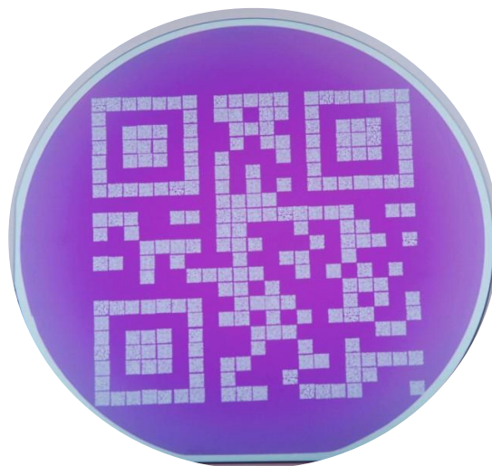
Figure 5: Tungsten Silicon-nitride gigayear storage technology developed at the MESA+ Institute for Nanotechnology (ExtremeTech, 2013).
